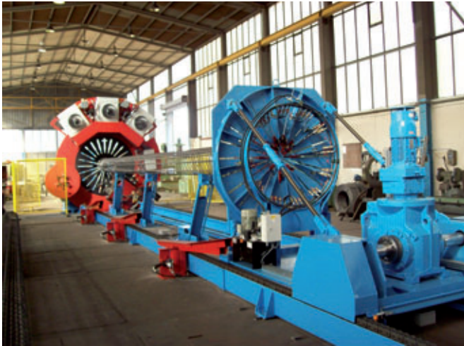
The cage welding machine from apilion can process up to 24 longitudinal bars with a max. thickness of 25 mm.
