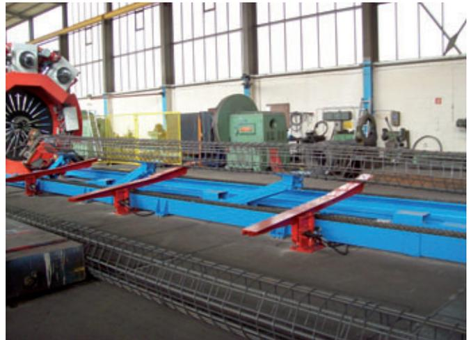
A finished reinforcing cage is fed to its further use by means of a lowerable cage support
