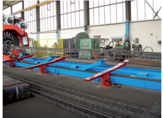
A finished reinforcing cage is fed to its further use by means of a lowerable cage support
